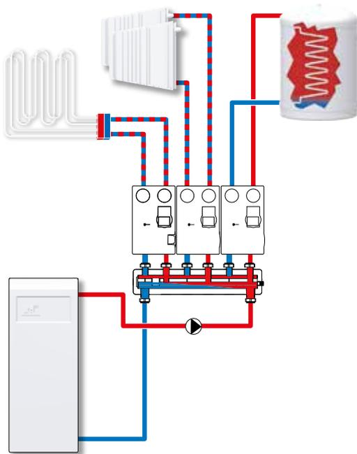
The primary function of the thermostatic mixing unit (GFx) is flow temperature control, mixing function. The Series GFx of circulation units are used in systems where the heating source is not equipped with a controller or a controller with limited functions. The circulation units series GFx are the perfect choice for applications where mixing function is required and temperature comfort is not the highest priority.
