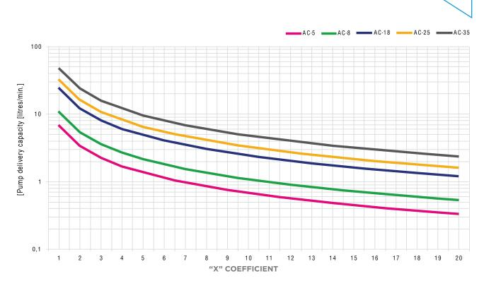
To make sizing easier, a chart has been drawn up to select the most appropriate accumulator according to both the working pressure and delivery criteria. Note that the chart is based on the following hypothesis: standard precharge and 15 pump starts per hour (see p. 27 to identify the "X" coefficient).
